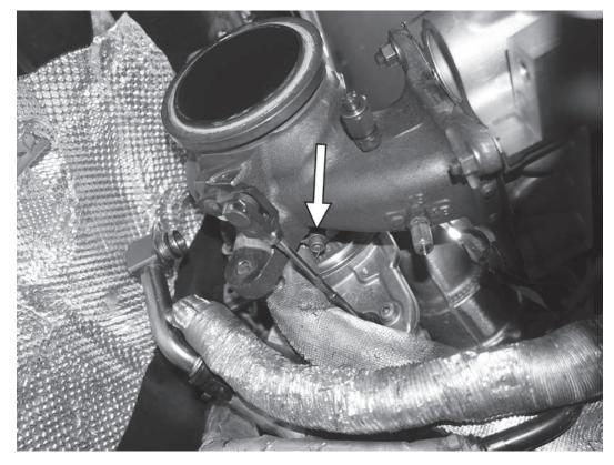
27) Remove the 8mm triple square from the oil drain line, and separate the line from the turbocharger.
