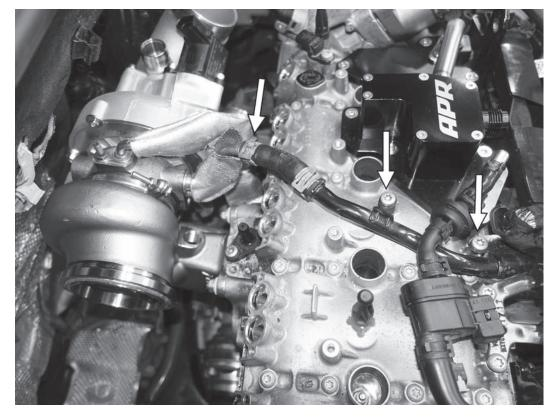
41) Reinstall the coolant pipe onto the top of the valve cover with the two T30 screws. Connect the hose to the turbo coolant feed pipe and secure with a spring clamp. Tighten the two T30 screws to 9Nm (80in-lbs).
