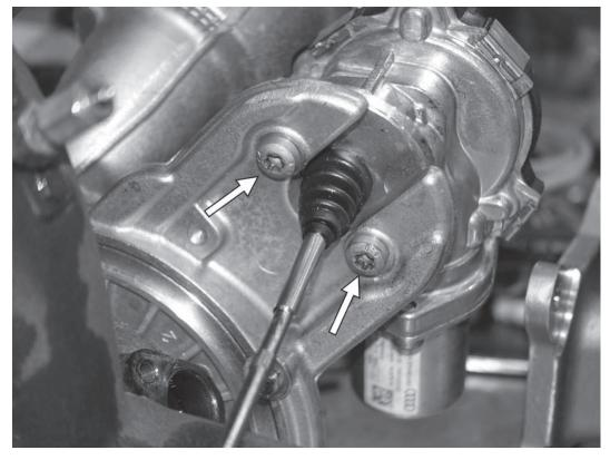
31) After noting the orientation of the wastegate solenoid on the stock turbocharger, loosen and remove the two T30 screws holding the wastegate actuator to the stock turbocharger.
