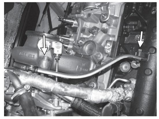
25) Remove the 6mm allen bolt from the top of the turbo support bracket. Remove the 13mm bolt from the bottom of the support bracket, and remove the bracket from the car.
