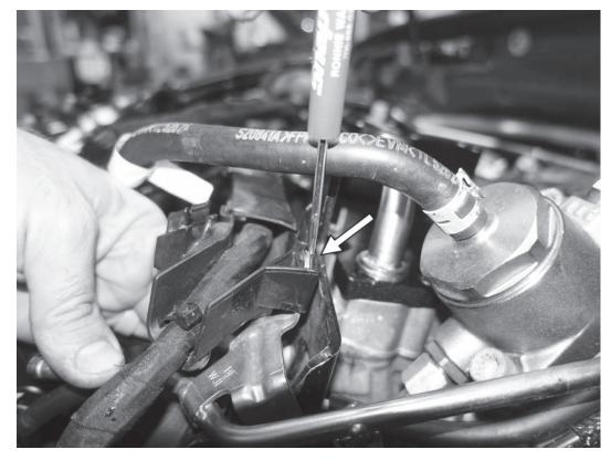
17) Separate the coolant pipe bracket from the wiring harness channel. Lift the wiring harness channel, and then remove the coolant pipe assembly from the car.
