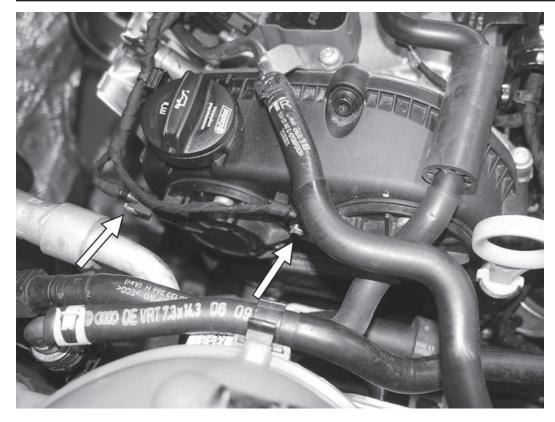
55) Reconnect the two electrical connectors to the two VVT camshaft solenoids.
