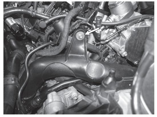
47) Reattach the side charge pipe with the T30 screw. Tighten the screw to 7Nm (62in-lbs).
