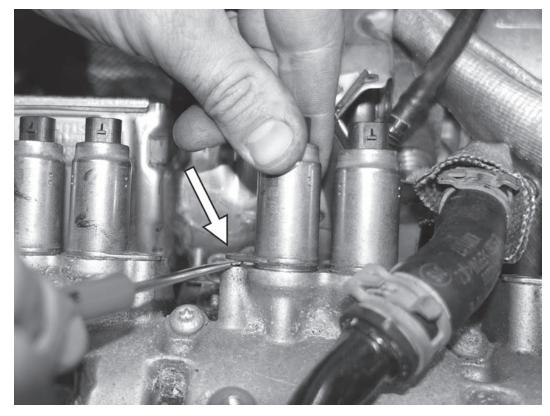
13) Using a small screwdriver, carefully lift on the flange of the valvelift solenoid while twisting the solenoid to remove it from the engine. Remove all eight valvelift solenoids.
