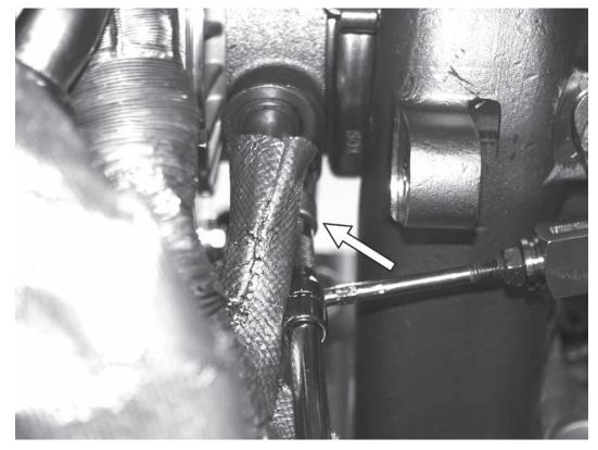
37) Replace the o-ring on the stock oil drain line with the new, supplied one. Install the drain line into the bottom of the turbocharger and tighten the 8mm triple square screw to 9Nm (80in-lbs).
