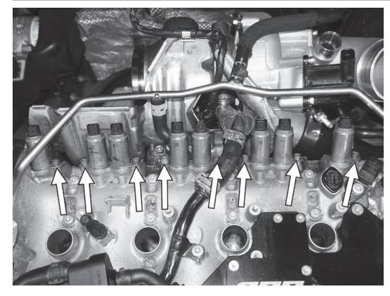
51) Reinstall the eight valvelift solenoids onto the back of the valve cover. Secure them with the eight T25 screws and tighten to 5Nm (44in-lbs).
