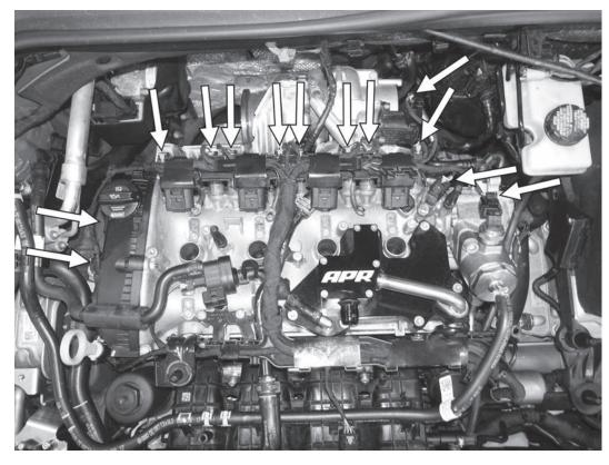
11) Disconnect the 8 electrical connectors on the valvelift solenoids, the one on the high pressure fuel pump, the one on the diverter valve, the one on the camshaft position sensor, and the two on each of the VVT cam solenoids. Lift the harness up and flip over towards the front of the engine.
