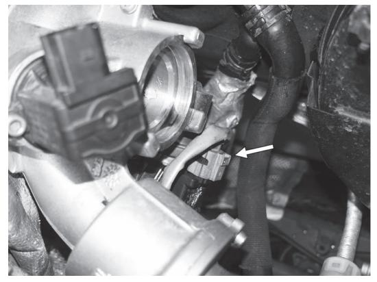
19) On the back of the turbocharger, disconnect the electrical connector to the wastegate actuator.
