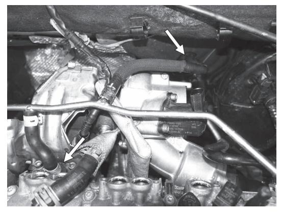
15) Remove the spring clamp and hose, and separate the coolant line from the back of the cylinder head. Remove the spring clamp and hose from the coolant line on top of the heater hose at the firewall.
