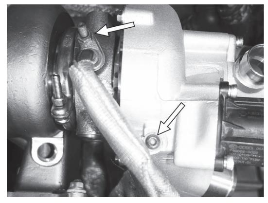
39) After replacing the o-ring on the oil feed line with the new, supplied one, install the oil feed line into the top of the APR turbo. Secure with the 10mm and 5mm triple square screws. Tighten both screws to 9Nm (80in-lbs).
