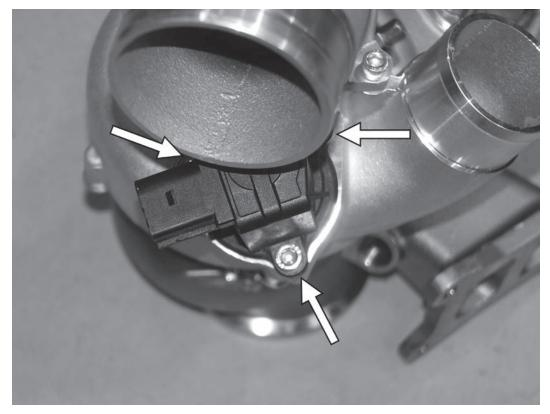
35) Install the diverter valve onto the APR turbo in the same orientation as it was on the stock turbo. Install the three 5mm allen screws and tighten them to 9Nm (80in-lbs).
