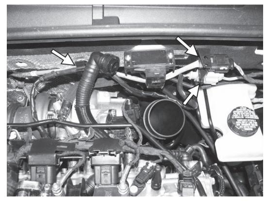
7) Separate both oxygen sensor electrical connectors from the mounting bracket on the firewall and disconnect the sensors. Separate the primary oxygen sensor wiring harness from all mounting connections.
