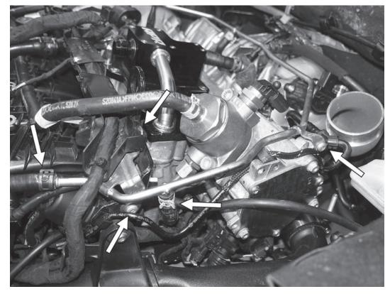
49) Place the factory upper coolant pipe assembly in the car. On the left side of the assembly, connect the hose to the front of the pipe and secure with the original spring clamp. Connect the pipe to the hose next to the side charge pipe. Reinstall the two T30 screws and tighten to 9Nm (80in-lbs). Finally, snap the wiring harness channel back onto the top of the coolant pipe bracket.
