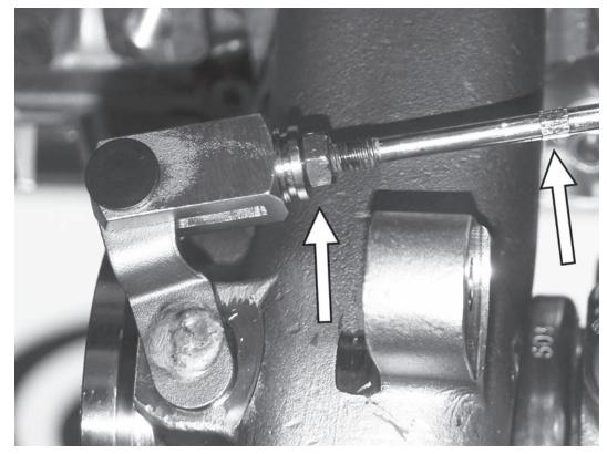
33) Thread the wastegate rod onto the wastegate flap by turning the wastegate rod. Do not change the location of the 10mm nut. Once seated, tighten the 10mm nut on the wastegate rod to 10Nm (88in-lbs). The overall length of the rod should not have changed from the stock turbocharger.
