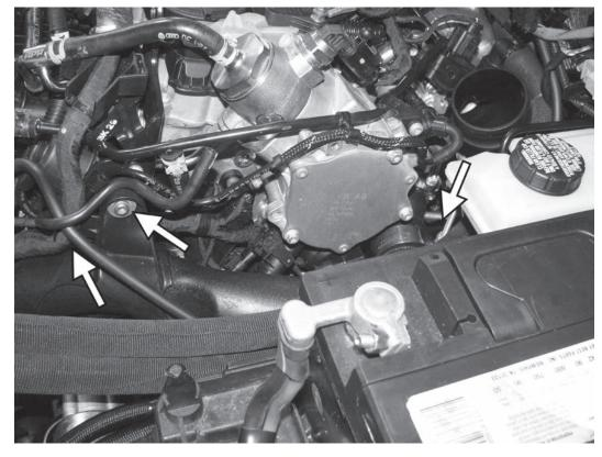
5) Remove the T30 screw from the side of the factory turbo outlet pipe. Unhook the wiring harness from the turbo outlet pipe. Remove the 7MM hose clamp connecting the turbo outlet pipe to the turbocharger outlet coupling hose. Finally, pull the turbo outlet pipe off and away from the turbocharger.
