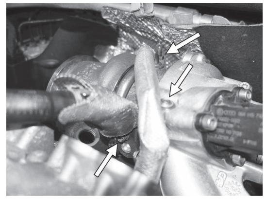
23) Remove the 5mm triple square screw holding the oil feed pipe to the top of the turbocharger. Remove the 10mm nut from the oil feed pipe on the back of the turbo, and carefully lift the pipe out of the top of the turbo. Remove the 8mm triple square screw from the coolant feed pipe on the front of the turbo.
