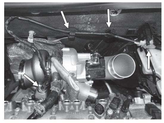
43) Reinstall the oxygen sensor into the turbo with an oxygen sensor socket. Tighten the oxygen sensor to 60Nm (44ft-lbs). Route the harness for the oxygen sensor roughly through the mounting clips on the firewall, and then reconnect the electrical connector to the wiring harness and mount the connector to the firewall.
