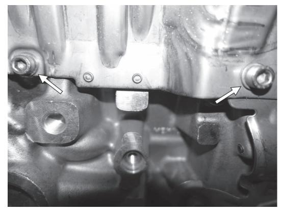
21) From the back of the heat shield, remove the two 5mm allen screws holding the heatshield to the back of the cylinder heat by the turbocharger. Remove the heat shield from the car.
