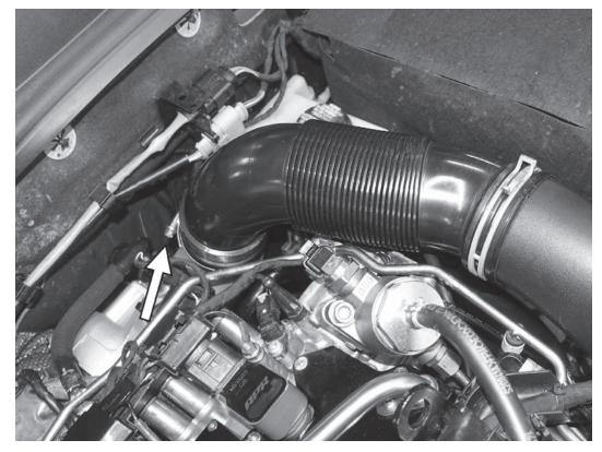
57) Reinstall the intake on the car. Tighten the 7mm screw on the clamp that connects the accordian inlet to the turbocharger. Reconnect the PCV hose to the turbo, or if equipped, the hoses to the APR catch can.
