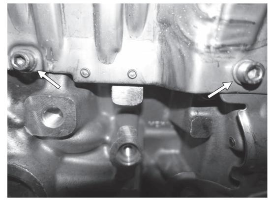
45) Reinstall the two 5mm allen screws on the back side of the heat shield. Tighten both screws to 9Nm (80in-lbs).
