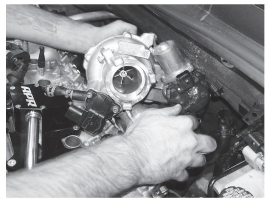
29) Carefully lift the turbocharger out from behind engine, making sure not to damage any surrounding components.
