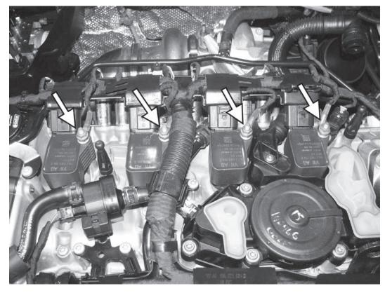
9) Remove the four 10mm nuts holding the grounding straps to the ignition coilpacks, and separate the grounding straps from the mounting posts. Once the ground straps are removed, remove the 10mm bolts holding the coilpacks in place.
