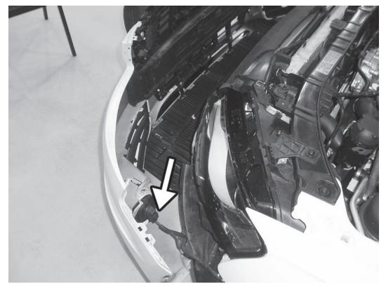
39) With an assistant, place the bumper cover back in front of the car. Reconnect the left and right fog light harness and bring the bumper back to its resting place on the core support.
