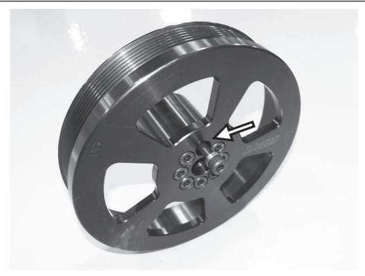
21) Install the 8x supplied bolts with washers into the APR crank pulley. Note that one of the holes on the APR pulley is slightly offset from the others.
