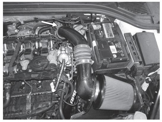
17) Place the intake back in the car, reconnecting the vacuum line to the bottom of it. Be sure all three mounting grommets are in place. Tighten the clamp holding the back of the intake to the turbocharger inlet. Finally, reinstall the engine cover.
