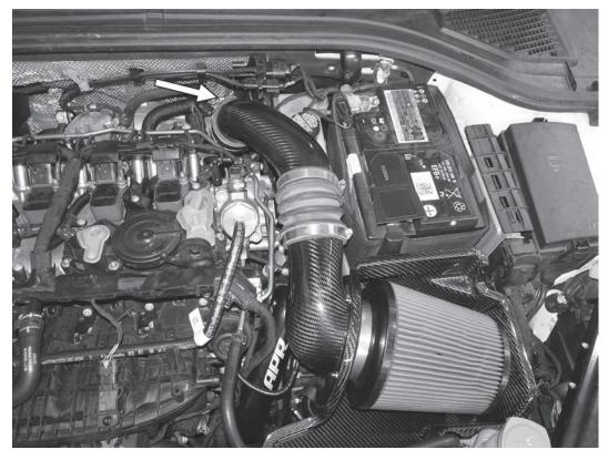
1) Raise the hood and remove the engine cover. Remove the intake from the turbo inlet as well as remove the airbox from the car. Use a rag to prevent anything from falling into the turbocharger.
