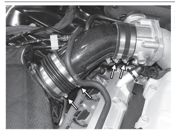
17) Rotate the throttle body end of the carbon fiber inlet hose assembly onto the throttle body. Adjust the hose clamps as needed, and tighten all four hose clamps.
