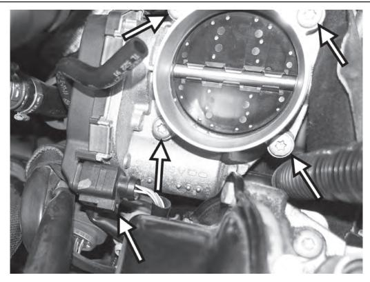
3) Disconnect the electrical connector to the throtlle body. Remove the four T30 bolts holding the throtlle body in place. These will not be reused. Remove the throttle body from the car.
