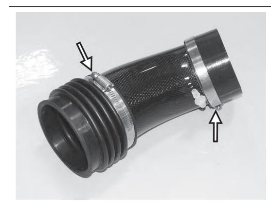
15) Install the silicone coupler on the end of the APR carbon fiber inlet tube with the supplied clamp. Install the accordian style coupler on the other end of the carbon fiber inlet tube and loosely secure with the supplied clamp.
