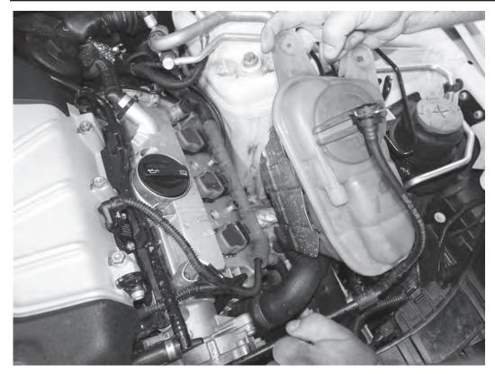
13) Lift the coolant bottle and bring forward to access the coilpacks on the left cylinder head. After removing the two T30 harness bolts and disconnecting the coilpacks, remove each coilpack one at a time. Change the spark plugs on each cylinder after properly gapping the spark plugs to  $.024" \pm .002"$ .
