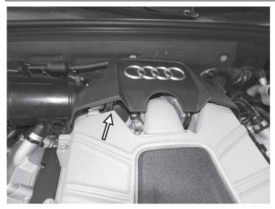
1) Remove the rear engine cover by carefully lifting up.
