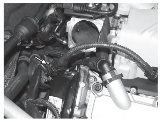
5) Connect the APR harness to the factory throttle body connector on the engine wiring harness.
