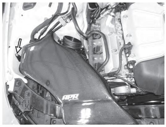
9) Lift the right side of the airbox from the clip on the inside of the fender.
