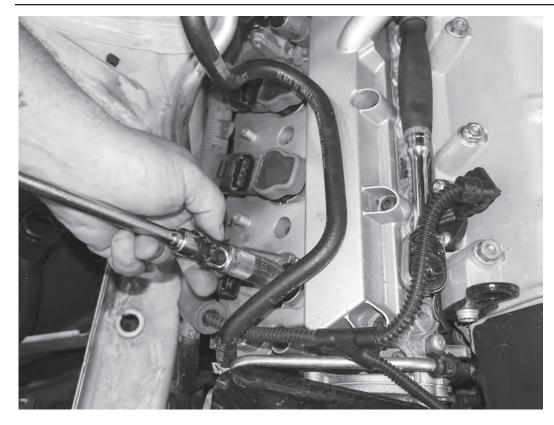
11) Remove the two T30 screws holding the coil pack wiring harness to the right cylinder head. Disconnect the electrical connectors from the coilpack and remove each coilpack one at a time. Change the spark plugs on each cylinder after properly gapping the spark plugsto.024"±.002".
