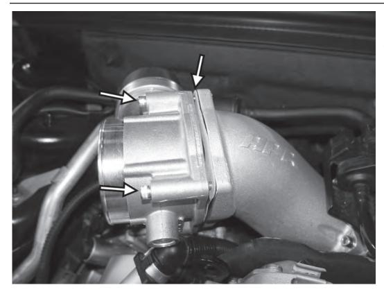
7) Install the APR throttle body with the supplied gasket to the cast APR inlet pipe as shown. Secure with the four bolts, threading them in by hand, and then torque to 88 in-lb (10Nm).
