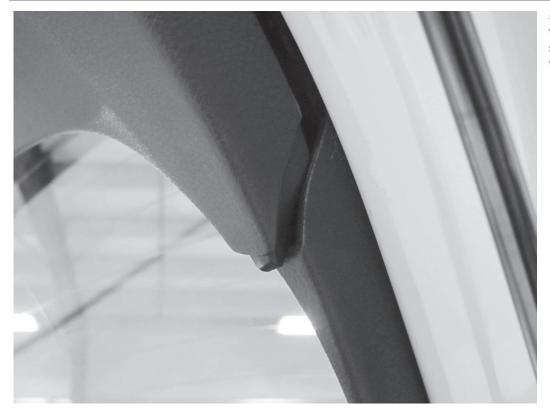
5) Note how the trim panel interfaces with the upper trim panel that surrounds the hatch glass. Remove the hatch trim panel from the car.
