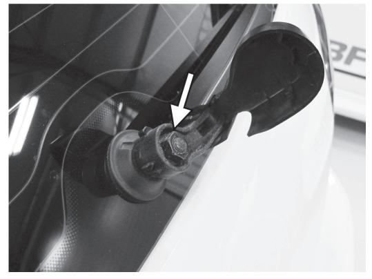
1) Carefully pry up the cover to the rear wiper by lifting the plastic cap from the left side of the wiper. Remove the 13mm nut holding the wiper in place.
