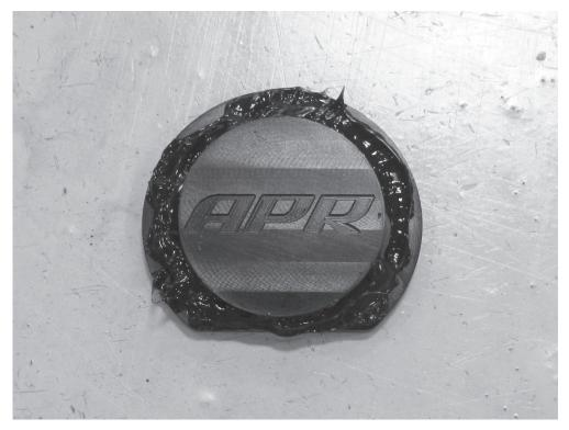
9) Clean the APR wiper delete with an alcohol based cleaner, and then apply the gasket material in a small bead around the wiper delete as shown.
