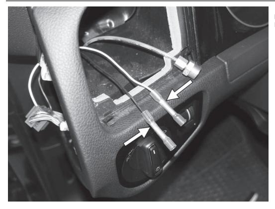
19) Crimp one side of the supplied butt connectors to both the white and black wires from the APR harness.
