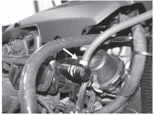
29) Install one end of the rubber hose to where you want to get a boost signal from, in this car an APR Boost Tap. Secure with one of the crimp clamps.
