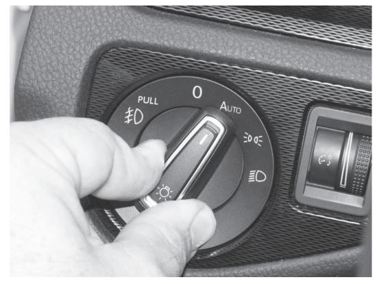
15) Remove the factory headlight switch. To do this, with the switch in the off position, simply push in on the switch, rotate the knob to the AUTO position. The switch can now be easily pulled away from the dash. Disconnect the red ten pin connector from the back of the switch. Do not turn on the ignition to the car with the switch disconnected.
