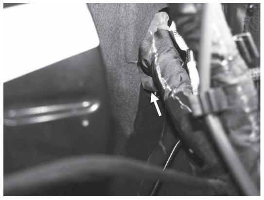
11) From under the hood on the firewall, locate where the main engine wiring harness goes through the firewall, just to the left of the factory brake booster. Either cut the end off the nipple under the wiring harness, or cut a small slit in the rubber grommet just below the wiring harness.
