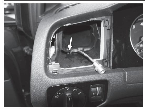
13) Install the end of the nylon hose without the fitting into the left vent opening, routing the hose down through the opening on the lower left side inside the vent hole.
