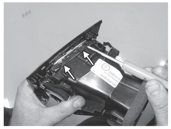
3) Using a small screwdriver, carefully unclip the eight clips holding the front trim plate to the vent housing. It is easiest to start with the two top clips, then do both sets of side clips, and then the bottom clips.
