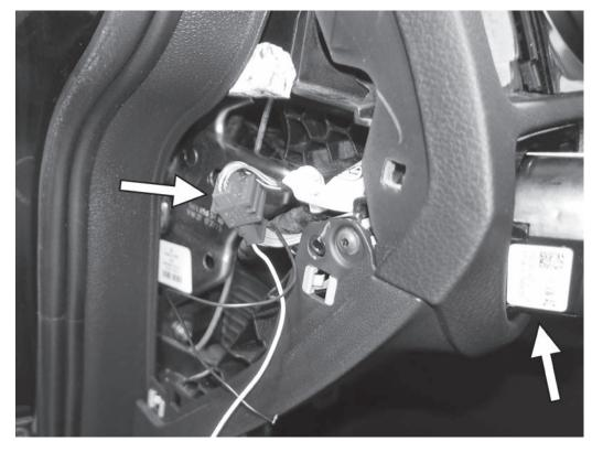
17) Pull the female connector of the APR harness with the factory harness attached back to the side of the dash panel while sliding the light switch back into the dash. Push the light switch back into the dash, turning the knob counterclockwise to the off position to lock the switch in the dash.
