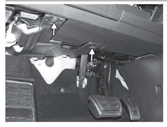
9) Remove the two T20 screws from the panel covering the bottom of the dash. Remove the panel by sliding it towards the back of the car.
