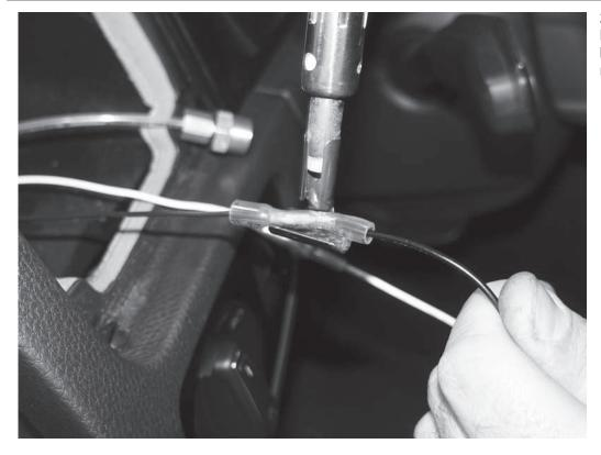
21) Use a heat gun or some other heat source to seal both ends of both butt connectors to the now connected wires.
