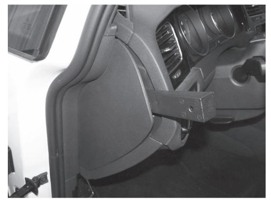
1) Using a plastic wedge or interior trim tool, remove the access panel inside the driver's door jam.
