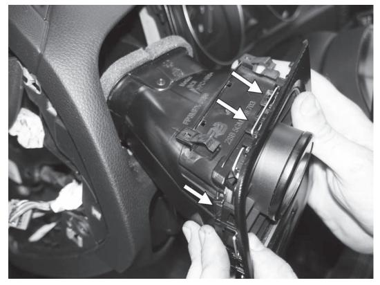
25) Slide the boost gauge with APR pod back into the back half of the factory air duct. Install the front face of the factory air duct, recliping all eight of the factory clips in place.
