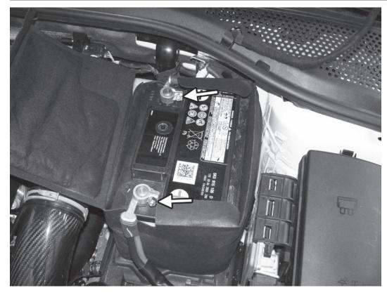
7) Raise the hood of the car and lift the cover to the battery. Disconnect first the negative connection and then the positive connection to the battery by loosening the 10mm screws on the battery terminals.
