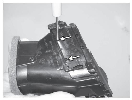
5) With a small screwdriver, press in on the four tabs (two on the top, two on the bottom) that hold the inner vent slats in place. Remove the inner vent slats from the vent housing.
