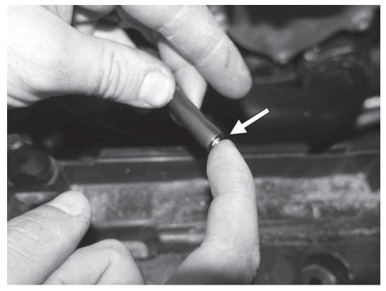
31) Put some spray lubricant into the end of the rubber hose and the install the brass pill into the rubber hose. Use a small screwdriver or pick to push the pill ~2-3" (50-75mm) into the rubber hose.
