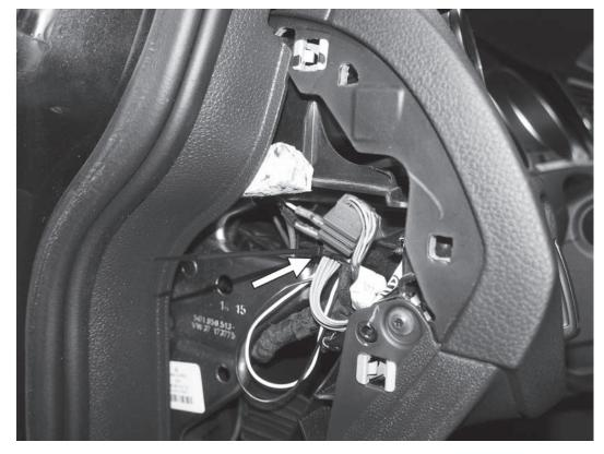
27) Neatly combine any excess wiring and secure with a cable tie in the area behind to the left of the dash. Replace the access panel onto the side of the dash.
