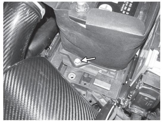
33) Slide the battery back on the battery tray. Slide the battery bracket back onto the battery, and reinstal the 13mm bolt to the battery hold down bracket.
