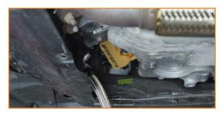
16. Feed the other end of the first line over the frame rail to the front of the driver-side wheel well.
