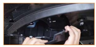
3. Disconnect the fog light on each side once you have access behind the splash shields. Depress the small tab at the end of the connector to separate the connection.
