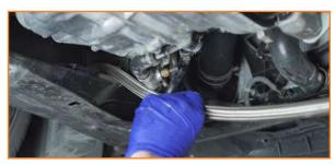
17. Install the 90° end on the shorter cooler line to the right-side port.
