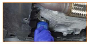
13. Install the sandwich plate using the hardware in your kit. Leave the bolt loose for now. (1x 1-1/16" bolt)
