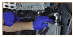
23. Install the shield bracket. Secure the top to the crash beam and the upper edge to the oil cooler. Torque the top bolt to the correct factory specifications.
