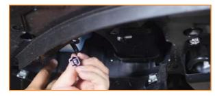
Remove the screws that secure the lower edges of the front bumper within the wheel well. (6x Phillips head screws)
