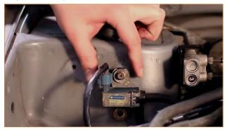
12. Disconnect the resistor near the passenger-side strut tower.
