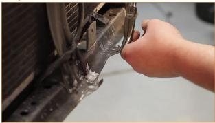
27. Position the supplied crash bar/ intercooler mounting bar bar where the stock crash beam was previously located, and secure with the stock hardware. (4x 14mm nuts, 2x 14mm bolts)
