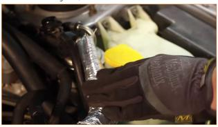
42. Secure the Mishimoto charge pipe onto the turbocharger outlet using the provided coupler and clamps. Snug the clamps, but do not fully tighten. You may need to reposition this pipe when installing the rest of the piping. Note: stock TD04 or VF series turbochargers will use the smaller outlet hose, whereas aftermarket 16G or 18G turbos will use the larger outlet hose. (2x clamps)
