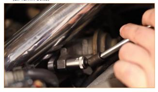
54. Attach the Mishimoto BPV hose from the BPV adapter to the port on the cold-side pipe, near the throttle body. Secure with the supplied worm-gear clamps. (2x worm-gear clamps)
