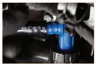
22. Locate the vapor hose with a 180° bend in your kit. Slip one of the provided worm-gear clamps over this end, and install it to the blue PCV elbow on the engine block. Then lead the other end of the hose behind the wiring harness and coolant hose; it should lie above the starter and hang over in front of the transmission when properly installed. Tip: Orient the clamp so that the adjustment nut is on the bottom for a flush installation. (1x worm-gear clamp)
