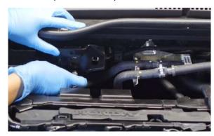
Release the fuel line from the two clips holding it in place. For the top one, use a flathead screwdriver to press in on the tabs clip before pulling it open.
