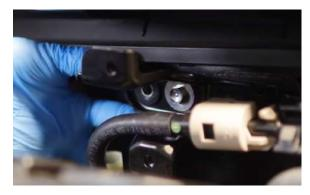
8. Install the Mishimoto catch can bracket behind the fuel line bracket and secure it with the original two bolts. (2x 10mm bolts)
