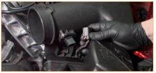
Remove the bolt that secures the airbox to the vehicle. (1x 10mm bolt)
