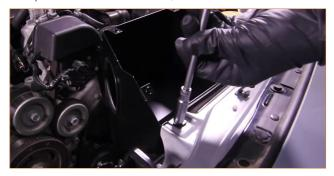
09. Lower the Mishimoto air filter into the airbox. Insert the MAF housing through the large hole on the airbox and into the air filter. When properly installed, the connector on the MAF should face toward the engine.
