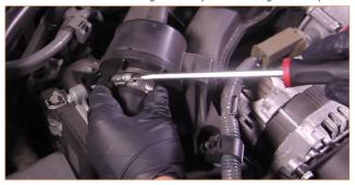
**14.** Install the Mishimoto airbox cover and secure it with the four provided Allen bolts. (4x 4mm Allen bolts)
