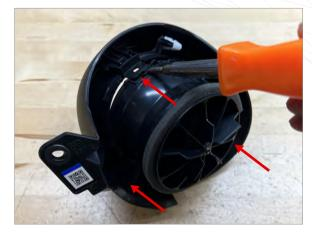
Use a screwdriver or pry tool to disconnect the 3 clips on the vent trim and then remove vent trim from housing
