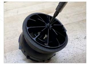
Remove screw from back of vent housing
