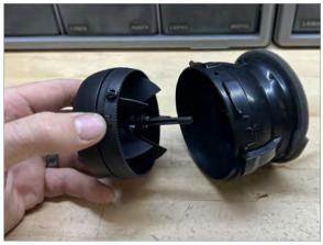
Remove internal mechanism from vent housing
