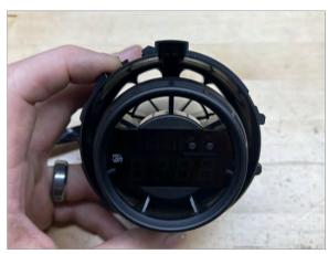
Install the display into the vent housing as shown, making sure tha the notch is at the top of the display
