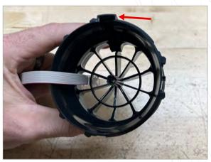
Insert display ribbon cable as shown.
