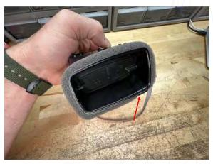
Fold ribbon cable around back of vent as shown
