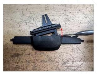
Remove the slider from the third slat by prying on side clips as shown
