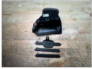
Remove the slats from the vent housing by pulling out on the left side of each slat
