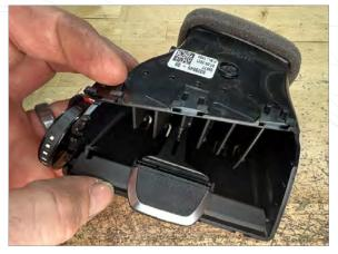
Reinstall bottom slat, making sure to line up vertical slat control fork as shown
