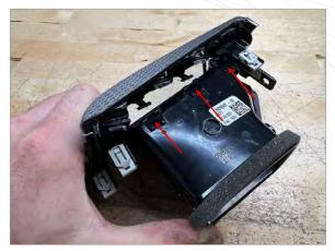
Remove trim from vent housing by releasing 3 clips on the top of the vent
