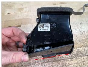
Install display by sliding right alignment pegs into corresponding holes in vent housing
