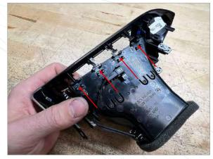
Then release 4 clips on the underside of the vent
