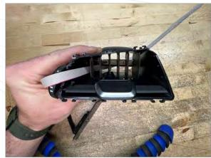
Route the ribbon cable between the leftmost vertical slat and the vent housing feeding it below the airflow control flap
