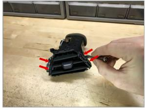
Release four clips to remove vent slat assembly
