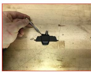
\*OPTIONAL Use a small screwdriver to remove the directional control fork.
