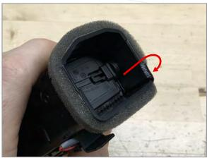
Fold the display cable around the back of the vent. Close air flap to hold display cable in place during installation
