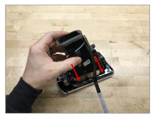
Reinstall trim to vent housing, ensuring that all clips are properly seated
