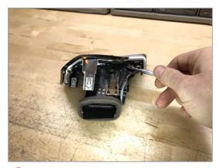
Use a small screwdriver or pry tool to release vent trim clips
