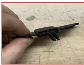
\*OPTIONAL Ensure that the fork extension is seated correctly as shown
