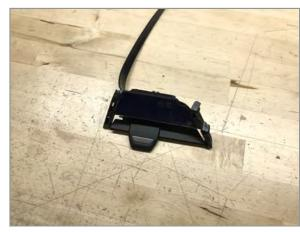
Install lower slat with or without slider and display into vent slat assembly
