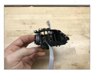
Feed the display cable through the vent to the left side of the furthest left vertical slat
