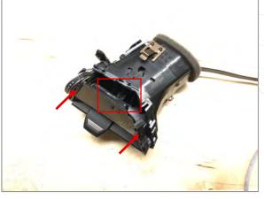
If reusing slider, make sure fork extension engages proper vertical slat. Slide slat assembly into vent housing
