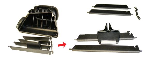
Remove the slats from the vent as shown. We will only be re-using the bottom 2 slats, so place the top 2 slats as well as the metal connector rod in a safe place in case you wish to return to stock.
