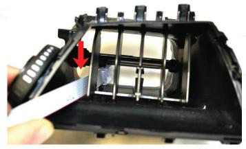
Insert the VIDI Display cable through the FAR LEFT side of the vent and out the back UNDER the open/close flap. Feed all the slack through.
