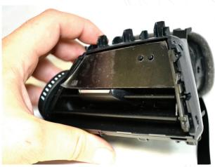
Replace the bottom slats and the vent slat holder on the far side, and insert the P3 VIDI display into the upper 4 holes where the 2 top slats were removed.
