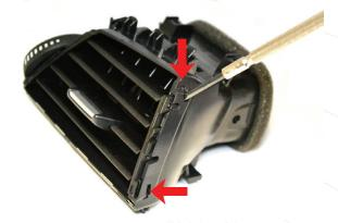
After removing the vent from the car, and removing the trim from the vent, it will look like the photo on the left. Using a flathead screwdriver, release the end of the slat holder on the side furthest from the open/close roller.
