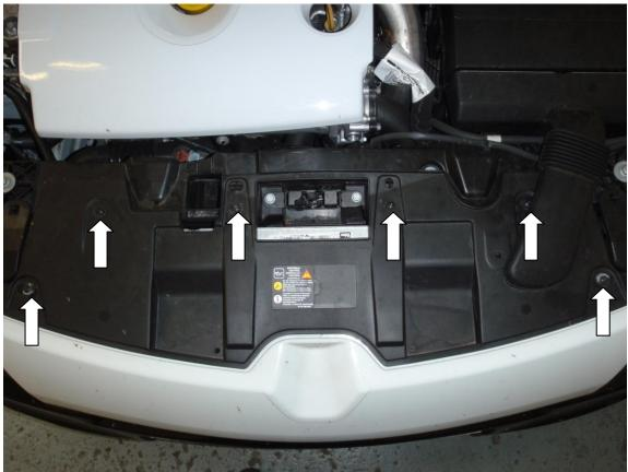
5. Grip the edges of the bumper where they meet the wing, and pull sharply to release it from the plastic clips along the edge.
