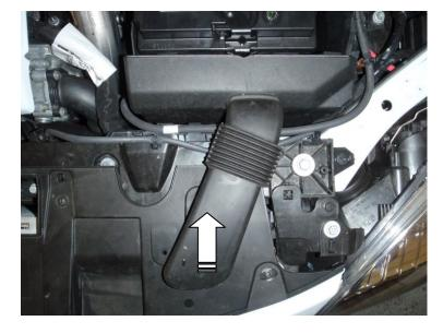
Pull the air feed upwards to release it from the top of the bumper, then pull the front section of the battery cover upwards to release it from the battery
