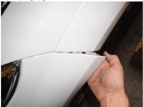
6. Lift the bumper forwards SLIGHTLY off the car, until you can access the electrical connector on the inside of the bumper on the passenger side (RHD) or drivers side (LHD). Ensure that the ignition is OFF, and detach the harness.
