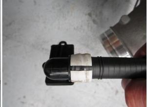
17. Fit the silicone hose to the turbo adaptor and fit the hose clamp into position ensuring it is pushed fully onto the adaptor and the hose clamp is tightened between the swage of the adaptor and the base.
