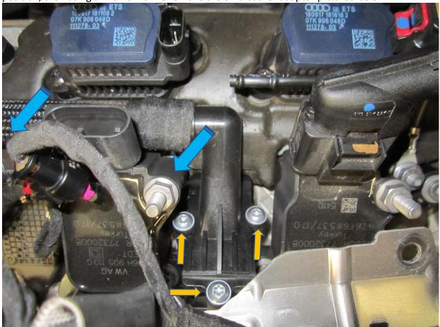
13. Using a T30 Torx Drive undo the two fasteners that hold the turbo elbow in situ. Access can be obtained from beneath the vehicle for one of the fasteners and from above for the other.
