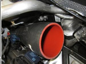
**18**. Refit the oil breather adaptor to the head and fit the barbed fitting supplied into the silicone elbow.
