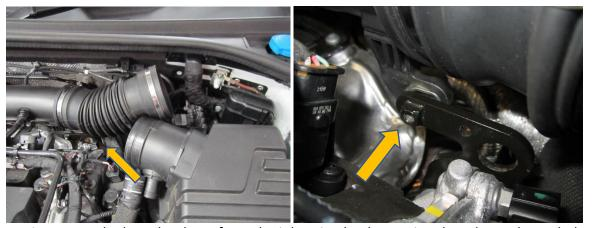
4. Disconnect the breather hose from the inlet pipe by depressing the tabs as shown below.
