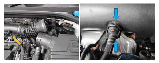
5. Using a hose clamp remover disconnect the sprung clamp that holds the inlet hose to the metal turbo inlet, then fully remove the inlet hose from situ.
