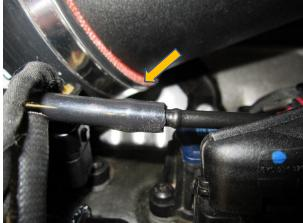
**16.** Remove the plastic pipe from the oil breather adaptor by either heating with a heat gun or by using a sharp knife to cut.
