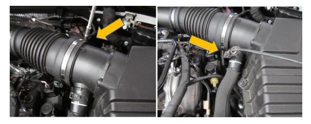
3. Remove the T25 fastener that holds the inlet pipe in position.
