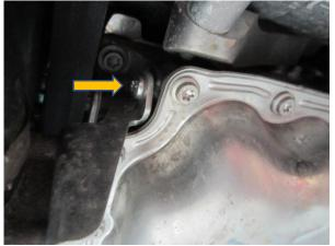
8. Undo the hose clamps that are still holding the boost pipe in situ.
