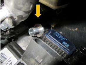
19. Fit the silicone hose from the oil breather adaptor on the head to the barbed fitting on the silicone elbow.
