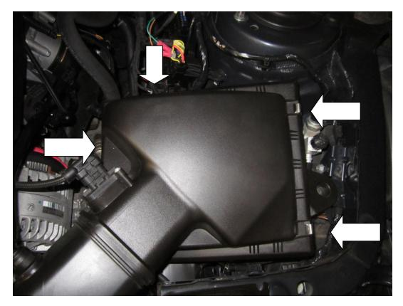
**13.** All that holds the induction pipe in place now is the rubber grommet in the center of the pipe. Simply pull the pipe towards you to release it, then place the pipe away from you on the engine so you can clearly see the wiring loom that enters near the front of the engine.
