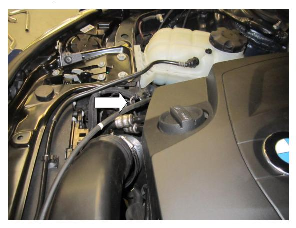
**15.** You now need to mount the solenoid provided with your new forge motorsport dump valve, we mounted it just behind the drivers light (RHD vehicle) where there is a spare hole available.
