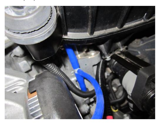
**22.** Route the smaller vacuum line across your engine next to the induction pipe you removed earlier, to the boost solenoid provided.
