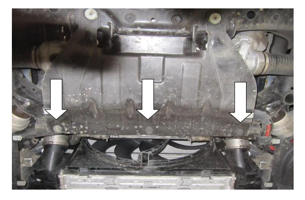
**3.** Remove the side undertrays in front of each wheel with your 8mm socket.
