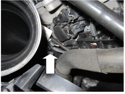
**14.** Once the loom has been identified simply pull it up from below the engine and re locate towards the back of the drivers side front light (on a RHD vehicle)
