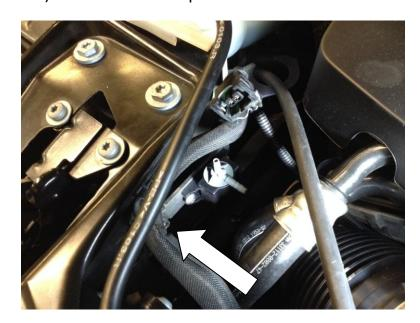
**16.** Next you must locate your vacuum source to make the valve work. Remove your engine cover by pulling it in a upwards, your vacuum will be taken from the pipe arrowed in the picture follow this down though the inlet manifold to where it connects to the vacum pump.
