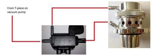
24. With the remaining vacuum line supplied, connect the upper and lower ports of the dump valve to the correct ports on the solenoid as shown. Double and triple check this as the valve will not function correctly if these are fitted the wrong way.
