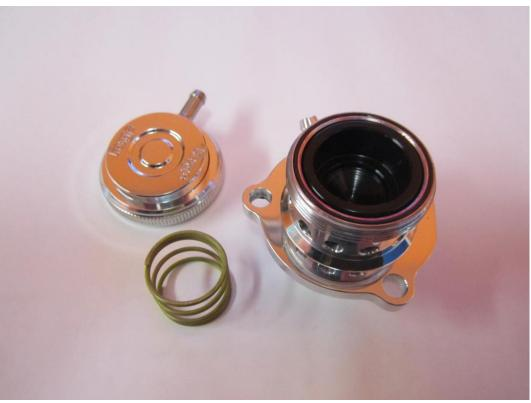
**8.** Before installing your forge motorsport dump valve make sure the orings are in place on the lower face as shown on the next page.
