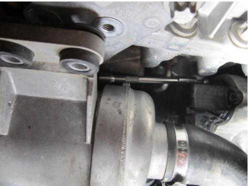
**7.** When fitting your forge motorsport valve you will need to remove the top section of the valve as this makes it easier to install. Rotate the top anti clockwise to remove.
