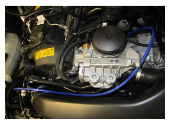
23. Connect this vacuum line to the solenoid on the port shown below
