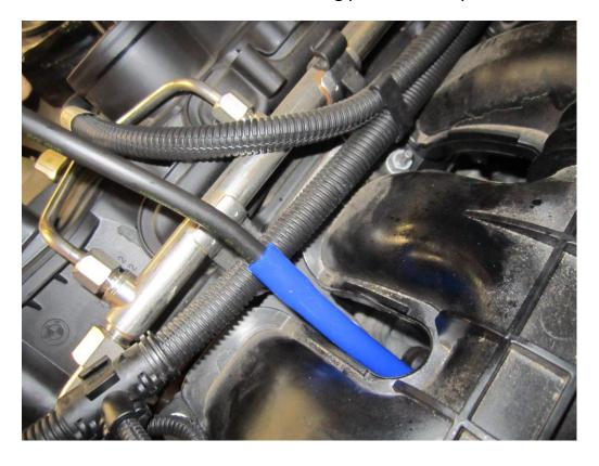
**21.** Now attach the smaller 3mm vacuum hose provided to the smaller outlet on the T piece then, attatch the shorter 6mm vacuum hose to the vacuum pump.
