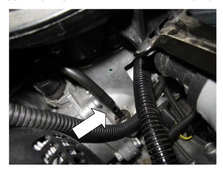
**18.** This pipe now needs to be cut down in order for it to still fit beneath the engine cover once the vacuum T piece has been installed. Pull the pipe up though the inlet manifold to make it easy for you to cut it, mark the pipe at 110mm from the end and with a sharp knife cut the pipe.
