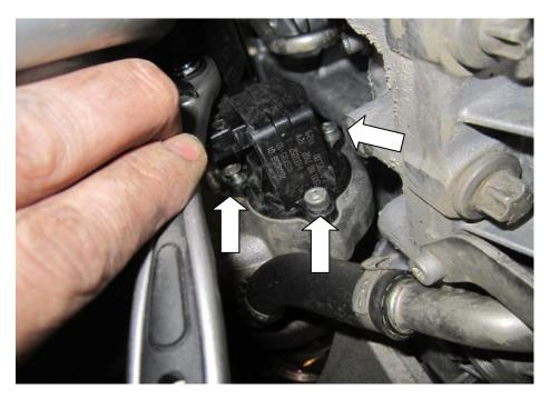
**6.** This next picture shows you the angle and position we took when undoing the fastener at the top of the valve. We placed our ratchet next to the rear of the radiator cowling and used two extensions to go inbetween the top of the water pump and pump housing, one extension was 150mm long the other was 100mm long.
