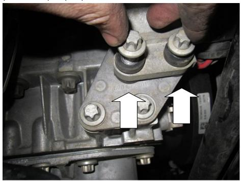
**5.** Remove the loom that conects to the top of the OE valve. Using your 6mm allen key undo the fasteners that hold it in place, this removal is very tricky we used various extensions to gain access to the fasteners .
