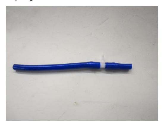
**20.**Now attatch the longer end to the pipe you have just cut making sure the vacum hose slides over the exsiting plastic tube by at least 20mm.
