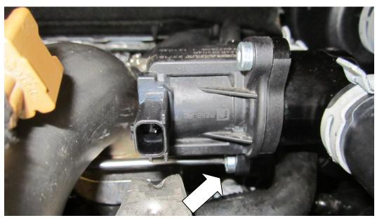
4. Using your hose clamp driver remove the two hose clamps that keep your valve attached to the induction pipe and turbo inlet.
