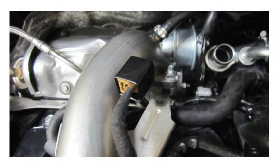
12.If your valve is the recirculating type connect the silicon pipe to where it has been blanked in step 10.
