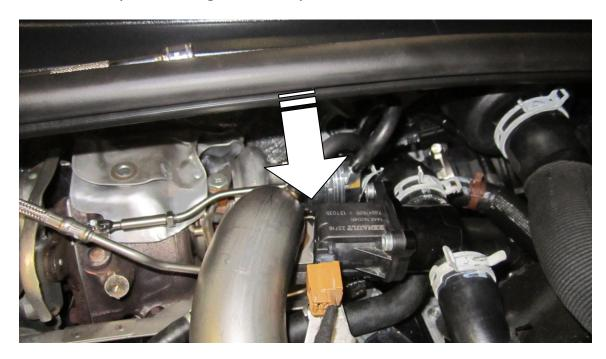
3. Using your T27 torx drive remove the two fasteners that hold the valve in place
