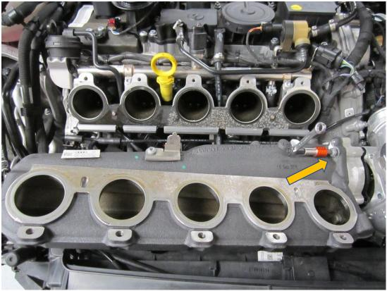
5. Attach the new Forge Motorsport high flow elbow to the throttle body ensuring the larger 82x3.5mm oring supplied is used for the new RS3 or TTRS with the DAZA Engine code. Use the 82x3.0mm O-Ring for the older engine.
