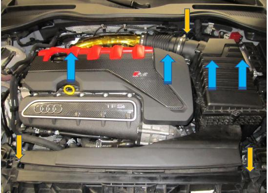
2. Unplug the MAP sensor, TPS sensor and t30 torx that hold the rocker cover bracket and the stock dumpvalve, then undo the hose clamp that holds the boost hose to the cast elbow.
