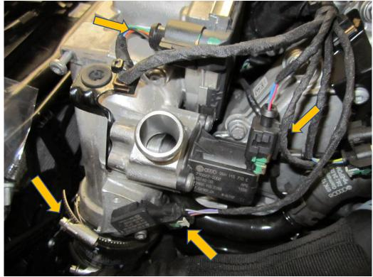
3. Remove three of the four T30 torx fasteners that hold the cast elbow to the throttle body and inlet manifold, using a 10mm socket undo the five bolts that hold the inlet manifold together.
