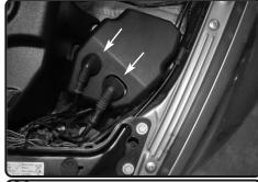
**23.** Re-install ballast cover, and reconnect both harness.
