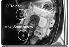
**22.** Install the ballast and position. Secure using oem bolt on top and nut, for bottom near headlight, use provided M6x35mm socket cap screw. Secure and tighten using allen key.
