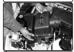
**8.** The air box cleaner is now pulled up and out of the way from the engine compartment.
