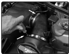
**24.** Tighten all clamps on the intake tube using 8mm nut driver.
