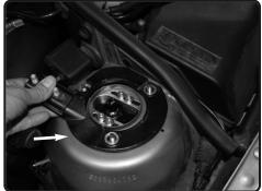
**26.** Re-install the strut tower plate.
