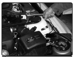
1. Loosen and remove two m12 flange nuts from each side of the strut tower bar. Remove the tower plate also, this will allow for more clearence.
