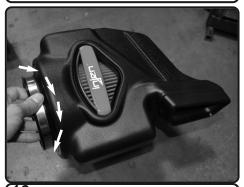
**16.** Once the twist lock filter is seated, rotate in either direction a 1/4" turn. Filter will lock into place.
