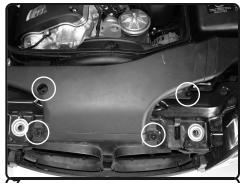
**7.** Removing the air scoop: Use a screwdriver to raise the center locking pin in the located on the clip. Remove all four plastic clips from the air scoop. Once you have removed the plastic clips, continue to remove the air scoop from the radiator shroud.
