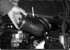
**9.** Continue to remove the plastic air intake duct connected to the oval throttle body.
