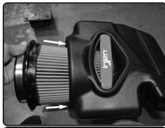
**15.** Install the twist lock filter to the air box.
