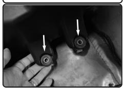
**20.** Install the grommets with cursh washers to the new injen air box.
