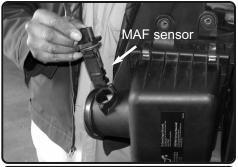
11. Loosen and remove the two screws on the mass air flow sensor. Pull the mass air flow sensor out of the sensor housing as shown above.
