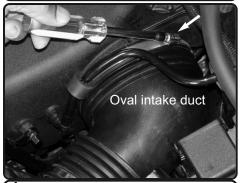
**4.** Loosen the clamp on the oval air intake duct located on the throttle body.
