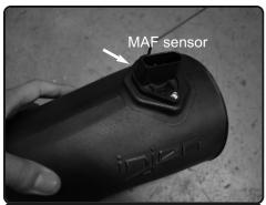
**12.** Install the MAF sensor into the new injen intake tube. Secure using provided M4 button head screws.
