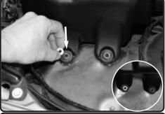
**21.** Place the nylon spacer provided to the first grommet closest to the headlight and set on top. This will allow clearance for the ballast cover.
