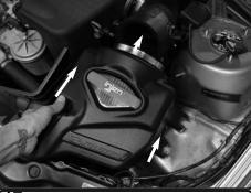
**17.** Install the air box assembly into position and connect the filter to the intake tube. Adjust and position if necesary.
