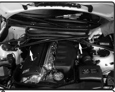
**2.** Once you have removed all four m12 flange nuts, continue to remove the strut tower bar.
