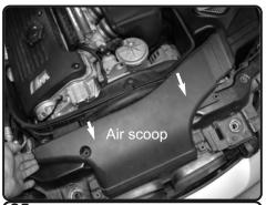
**25.** Re install the air scoop and secure from step 7.
