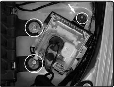
7. Loosen and remove the two m10 bolts and the m10 flange nut. Lift up and remove the Zenon ballast out of the way, this will allow you to remove the air box cleaner. Set Ballast to the side. Save 1 bolt and nut for later install.
