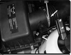
**5.** Loosen the clamp located on the lower air intake duct connected to the mass air flow sensor.
