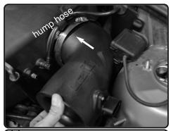
**14.** Install the intake tube and positon the tube to the hump hose on the plenum. Do not tighten.
