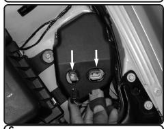
**6.** Press upper tabs on the electrical harness clips that connects to the Zenon ballast. Once you have disconnected the electrical harness clips, continue to remove the ballast cover.
