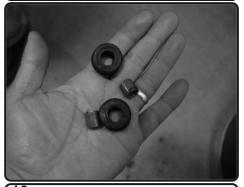
**19.** Remove the OEM grommets and crush washers from the stock air box. This will be used on the new injen air box.
