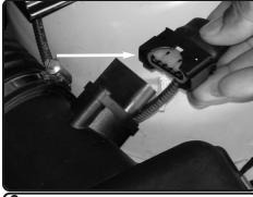
Press the side tabs on the electrical sensor harness and pull the harness away from the mass air flow sensor.
