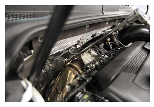
**Step 2:** Lift the vehicle on jackstands or hoist. Using a 22mm wrench or O2 sensor removal tool, remove the O2 sensor from the downpipe.
