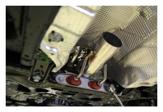
**Step 10:** Slide the included accuseal exhaust clamp over the downpipe and install the secondary pipe. Adjust to correct length for the oem exhaust clamp to slip over. Tighten down both clamps.
