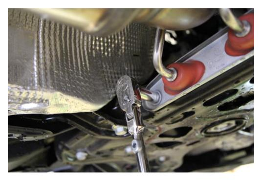
**Step 7:** Using the 13mm socket, remove the 2 bolts holding the downpipe bracket to the engine block. Pull the downpipe free of the car.
