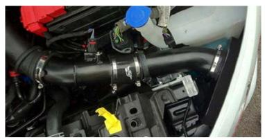
When you are satisfied that everything is positioned correctly, you can tighten up the hose clips remembering not to over tighten them as this could damage both the pipe work and filter neck. With the pipe work in place, attach the rubber strap to the bracket then retrieve the MAF from its safe place and reconnect the sensor. Plug the wiring connector back into the headlamp before dropping the unit into place, remembering to centre the
