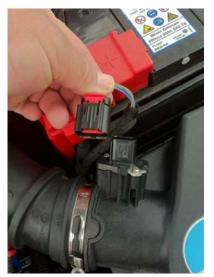
The first step in fitting your induction kit is to remove the stock air-box. Gently disconnect the MAF sensor, remembering to depress the red safety latch. This will allow the plug to be removed correctly, before loosening off the hose clip that connects the air-box lid to the inlet.
