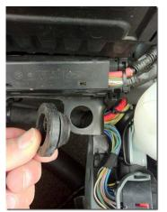
While you still have a big open space, it's a good idea to fit the bracket that holds the wiring harness in place. Remove the right
