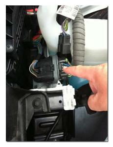
Down on the chassis leg, there is a large wiring loom connector attached to a plastic moulding. This is fixed on with a one-way catch and is awkward to remove. There is no need to split the loom at the connector, just remove it from the chassis leg.
