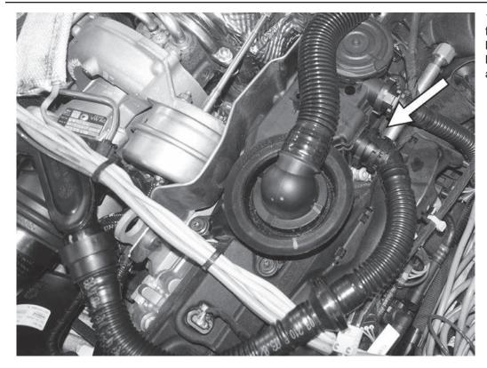
13) Unplug the front PCV connector from the left side of the engine, just behind the oil fill tube. Press in on both sides of the connector and pull away from the engine.
