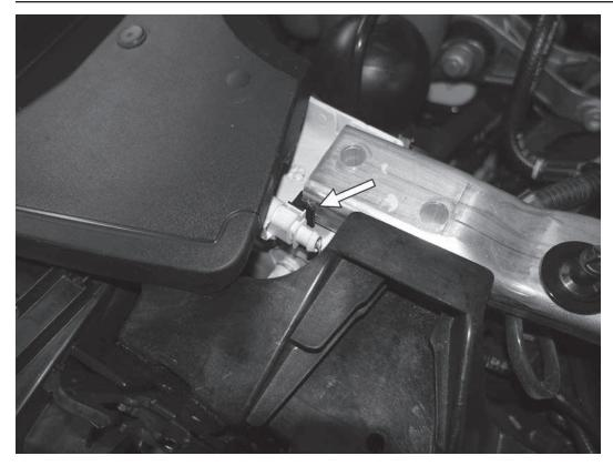
29) Reattach the crash sensor electrical connector to the right side of the front crossbrace, making sure to not unplug the electrical connector.
