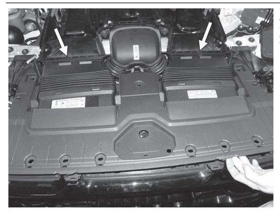
7) Lift up on the front of the front cover, then pull the cover forward. Separate the cover where the accordian ducts meet the bottom of the airbox.
