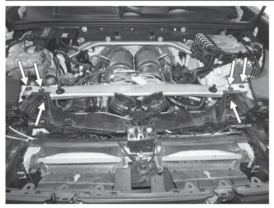
11) Remove the six T30 screws holding the front crossbrace in the engine compartment.
