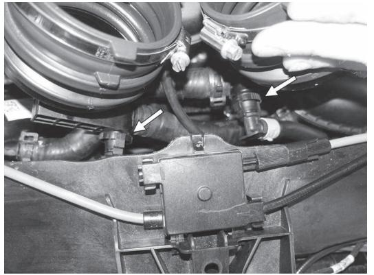
15) Disconnect the two quick disconnect fittings on the front of each front turbo inlet hose.
