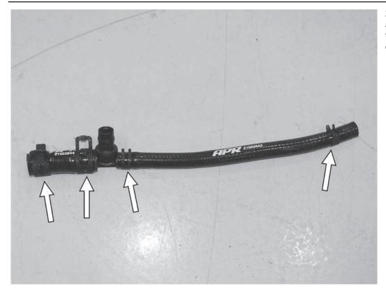
21) Build two of the shown hose assemblies with the APR EVAP suction jet, two large and two small hose clamps and hose.
