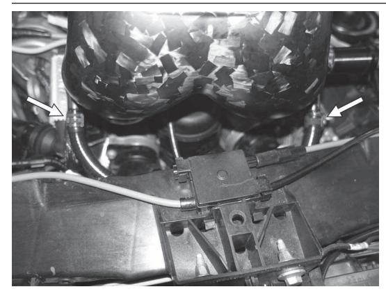
27) Connect the lines from the APR hose assemblies onto the ports on the front of the turbo inlet pipe. Adjust the routing of the hoses so that there are no kinks in the hoses. The hoses will cross from side to side; the hose assembly from the right side of the engine connects to the left port on the turbo inlet pipe, and the hose from the left side of the engine connects to the turbo inlet pipe.
