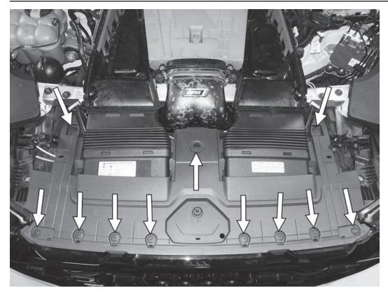
37) Reinstall the eleven push pin connectors holding the front panel to the car. Make sure to install the pins in the same location as they were originally.
