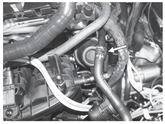
11) If not installing the APR coolant hose, tuck the factory coolant line under the APR airbox once installed, and skip to step 15. On the coolant line that ran over the airbox inlet scoop, remove the spring clamp that connects the hose to the metal pipe by the intake manifold. Remove the line from the pipe using a pick to loosen it. Use the supplied rubber cap over the metal pipe to keep the car from losing too much coolant.
