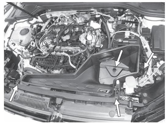
17) Place the APR airbox base in the car, pushing the installed grommets onto the factory airbox mounting posts. Make sure the sides of the APR airbox base aligns with the mounting tabs the factory airbox inlet base connected to the radiator core support. Ensure the APR airbox base is fully seated on the factory airbox mounting posts.
