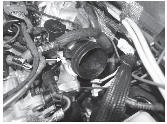
19) Lubricate and then install the supplied o-ring on the APR turbo inlet adapter. Push the inlet adapter into the turbo, ensuring the tab on the adapter seats into the slot on the turbo. The inlet adapter will be about 20° off clockwise from where it will finally sit.
