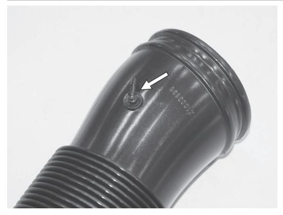
23) Install the supplied 90° barbed fitting into the rubber grommet in the APR inlet pipe.
