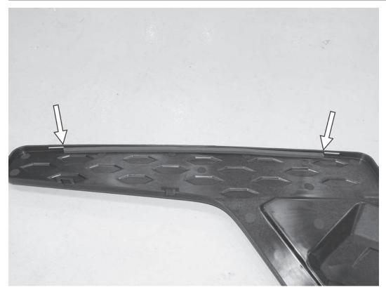
27) If installing the APR airbox lid, install the supplied foam tape on the bottom side of the airbox lid, between the two tab slots that are in the front of the lid.
