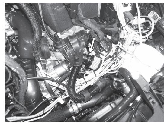
15) If equipped, clip the APR secondary air filter into the end of the factory secondard air connection, and then tuck the filter and pipe under the airbox mount. Secure the pipe with the supplied cable tie.
