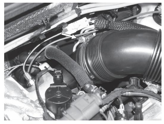
7) Loosen the 7mm screw on the clamp that connects the airbox inlet pipe to the turbocharger. Once loose, firmly pull the inlet pipe off the turbo inlet.
