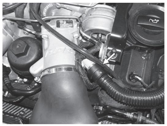
19) Reconnect the PCV valve to the right APR cast turbo inlet pipe by pressing it in place.
