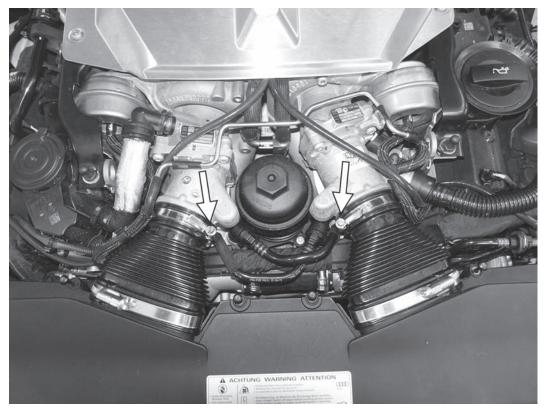
3) Loosen the two 7mm hose clamps holding the accordian hoses to the cast turbo inlets.
