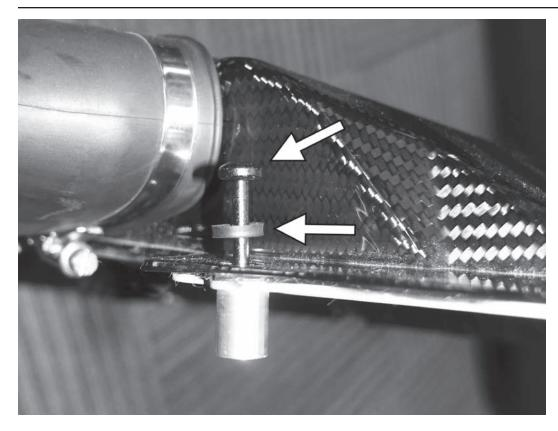
13) Completely unscrew the eleven T25 screws from the OEM airbox lid. Using the plastic washers, install the eleven screws onto the APR carbon fiber airbox lid.
