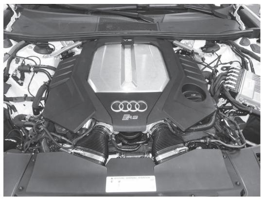
1) Raise the hood and remove the engine cover by lifting up on all four corners of the cover.
