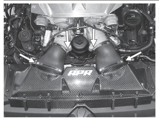
17) Adjust and tighten the clamps on the APR inlet hoses to the APR cast turbo inlet pipes, ensuring everything is seated unstressed. Torque all four 7mm screw clamps on both ends of the inlet hoses to 7Nm(62in-lbs).
