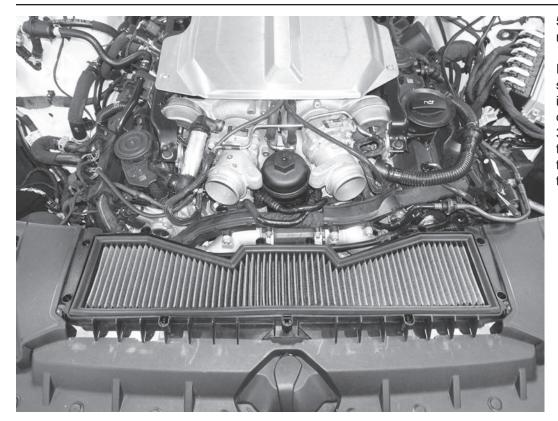
5) Remove the OEM air filter and replace with the APR air filter.
