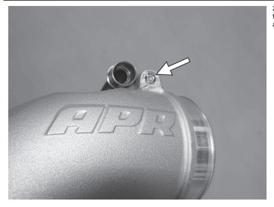
25) Remove the 4mm allen screw from the APR turbo inlet pipe and set aside for use later.
