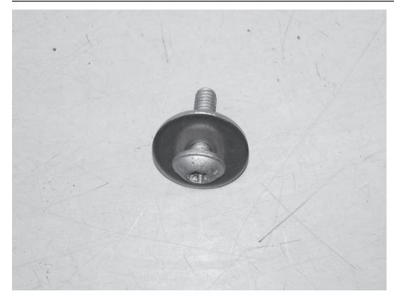
45) Take the T30 screw that held the stock intake to the back of the cylinder head, and add the supplied large washer.
