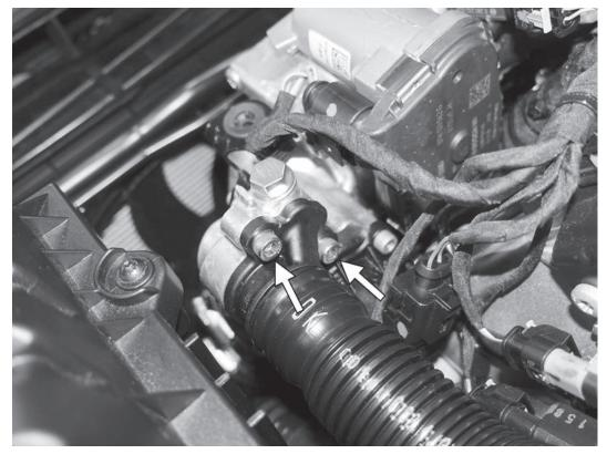
7) If equipped, remove the two fasteners holding the front of the accordian inlet pipe to the throttle body inlet tube. Remove the accordian pipe from the inlet tube.
