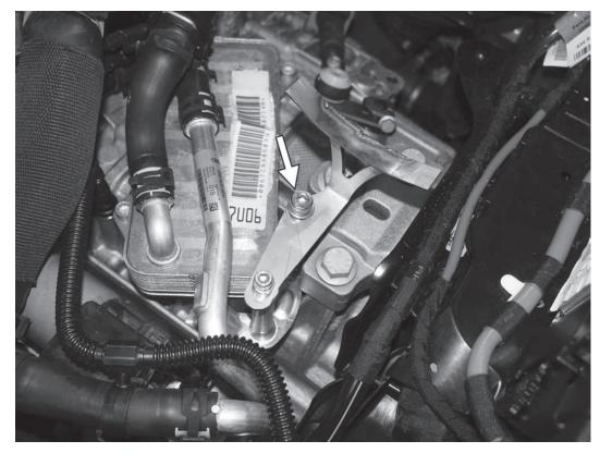
13) Remove the 10mm triple square screw from the back of the same mounting bracket, and loosely install the bigger diameter screw from the previously made APR assembly.
