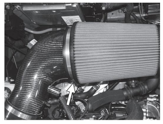
21) Secure the air filter to the APR intake and the bracket by tightening it to 10 in-lb (1.2Nm).
