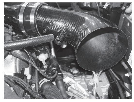
15) Loosely place the APR carbon fiber intake assembly in the car, loosely connecting the silicone hose to the APR inlet tube.
