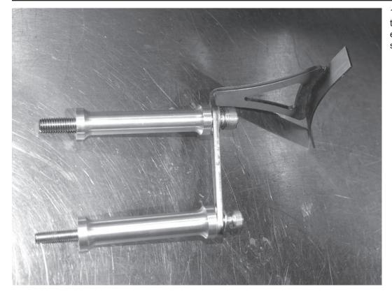
11) Make the following assembly with the APR bracket, screws, and spacers. Note that the smaller diameter screw is on the end of the bracket.
