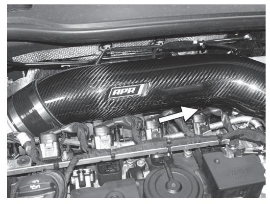
19) It may be necessary to adjust the APR inlet tube for desired fitment of the APR intake. Loosen the T30 screw on the intake and make adjustments if needed.
