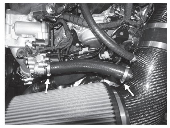
23) If installing on a car that had an accordian inlet pipe, install the supplied hose, trimming the length if necessary, and secure with the supplied hose clamps.
