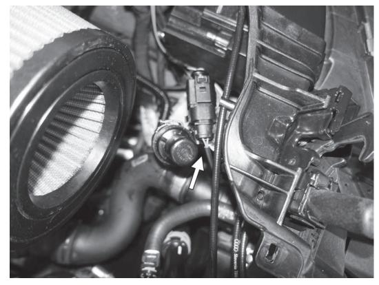
25) If equipped, attach the factory transmission vent to the back side of the headlight by pushing the mounting clip onto any straight piece of plastic.
