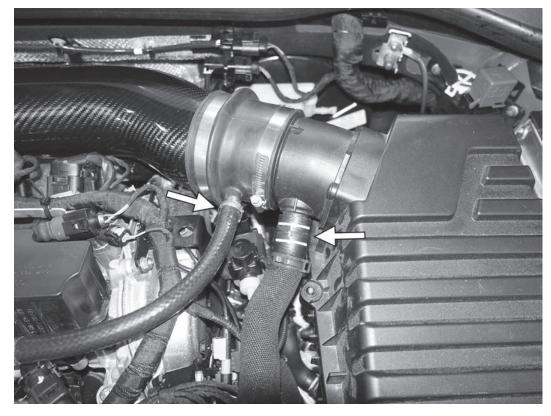
3) Disconnect the spring clamp from the larger of the two hoses on the back of the airbox and disconnect the hose. Remove the ear clamp from hose side of the smaller N80 valve hose, and disconnect the hose from the back of the airbox. On some cars without a spring clamp, remove the two 5mm allen screws holding the larger hose in place.
