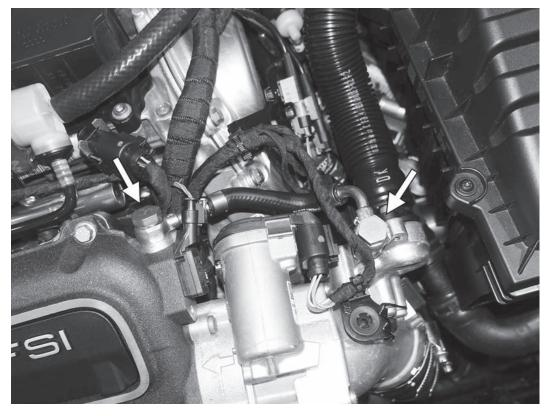
5) If equipped, remove the two 17mm banjo bolts connecting the tube between the intake manifold and the throttle body inlet tube. Remove the hose assembly with the sealing washers.
