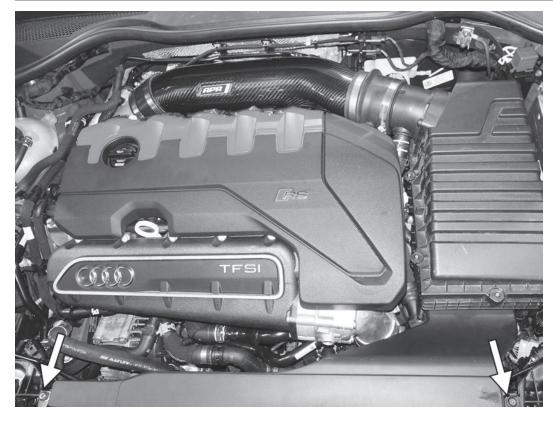
1) Raise the hood of the car, and remove the engine cover by lifting up on each of the four corners.
