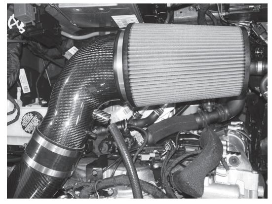
17) Loosely install the filter onto the end of the APR carbon fiber intake, making sure the APR bracket sits between the outside of the air filter and the large hose clamp.
