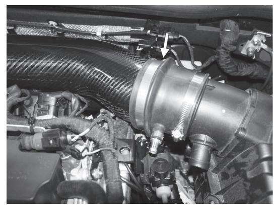
9) Loosen the screw clamp holding the airbox elbow to the APR rear inlet pipe. Lift up on the airbox assembly to separate it from its rubber mounting posts and remove the airbox assembly from the car.
