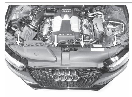
21) Reinstall the cover over the radiator, making sure the front of the cover connects back correctly to the top of the bumper cover. Install the four reset pins in the holes of the upper radiator cover, and then push down on the center portion of the pin to lock the cover in place.
