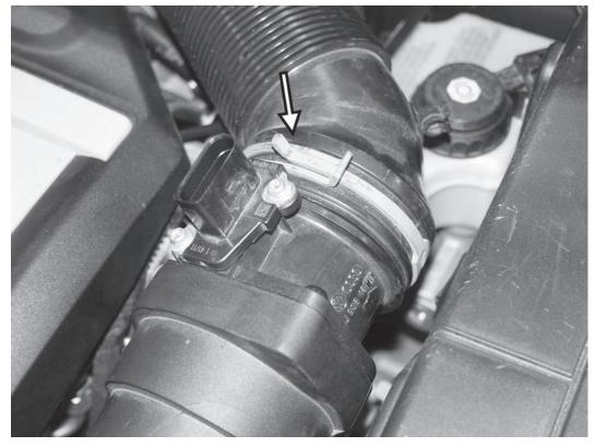
5) Squeeze the hose clamp holding the accordian inlet elbow to the back side of the MAF sensor, and slide the clamp off the MAF sensor. Separate the inlet elbow from the MAF sensor.
