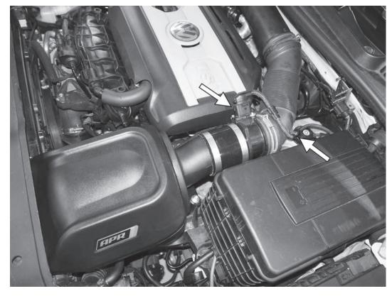
17) Reconnect the electrical connector to the MAF sensor. Reclip the MAF sensor wiring harness back onto the accordian inlet tube.
