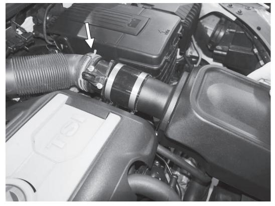
13) Loosely install the APR intake assembly in the car. Attach the according inlet elbow to the back of the MAF sensor housing and secure with the factory spring clamp.
