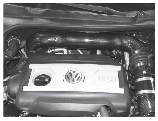
15) Reinstall the engine cover by pushing the four corners down onto the mounting posts on top of the engine.
