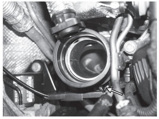
5) Remove the lower spring clamp from the couple that held the rear intake pipe to the turbo inlet. Remove the coupler with the spring clamp. Be careful not to drop anything into the turbo inlet.
