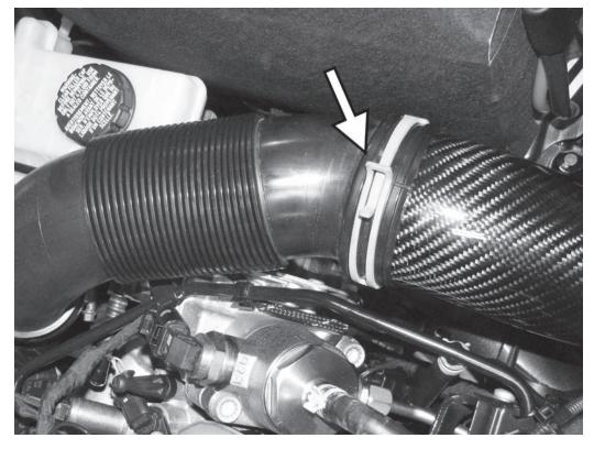
1) Remove the factory engine cover by lifting up on the corners of the cover and lifting up. Remove the spring clamp holding the back of the APR intake to the factory accordian inlet tube by sliding the clamp over the inlet tube.
