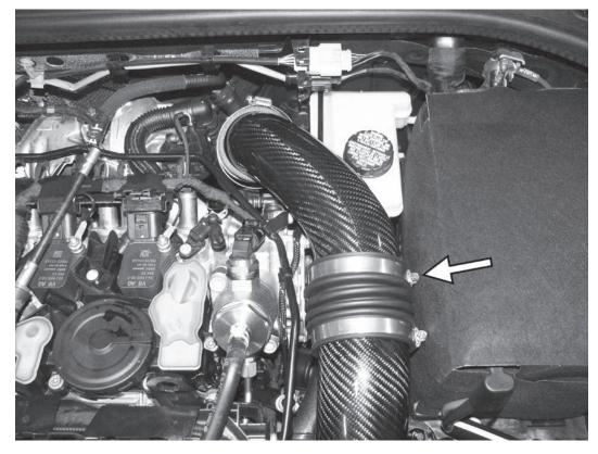
5) Install the APR Stage 2 pipe between the two couplers. Secure the front side of the pipe to the APR accordian coupler with one of the supplied 8mm hose clamps.
