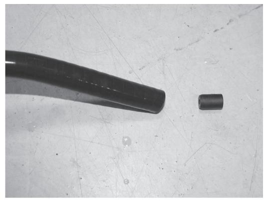
5) Install the one way check valve in the end of the APR hose that goes to the engine. Be sure to install the check valve in the same orientation as it was in the stock coolant hose.
