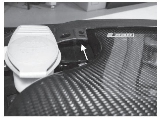
7) Carefully loosely place the APR intake back in the car. Connect the intake into the slot on the back side of the core support, and then slide the intake towards the right side of the car to lock it in place. Install the screw holding the APR intake to the back side of the radiator core support.
