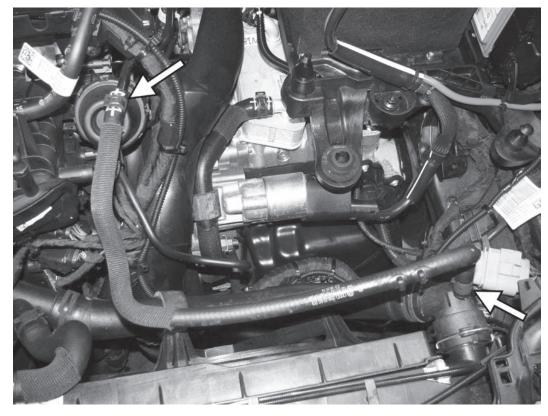
3) Remove the factory coolant hose from both the engine and the upper radiator connection. Be careful not to break the plastic barbed fitting on top of the radiator connection. Use the supplied rubber caps to keep coolant from pouring out.
