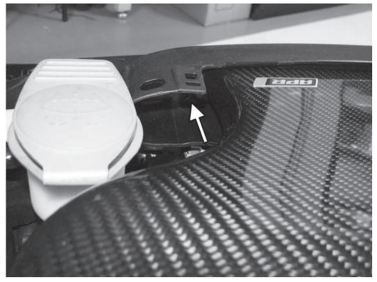
1) Once making sure the engine is cold, remove the cap from the factory coolant reservoir. Remove the screw holding the APR intake to the back side of the radiator core support. Slide the intake towards the left side of the car to separate it from the core support.
