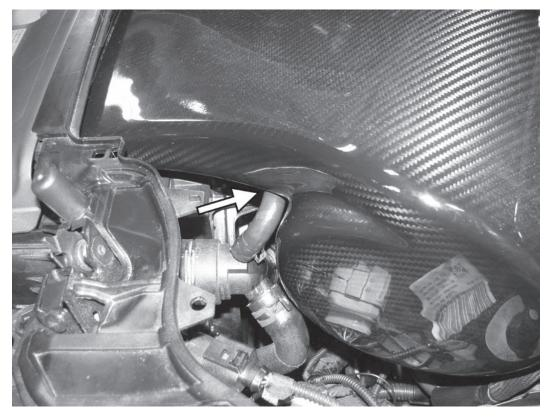
9) Ensure the new coolant hose is not kinked underneath the bottom of the APR intake.
