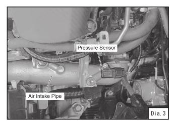
(9) Remove 2 bolts and loosen hose clamps to remove the air intake pipe. (Dia. 3, 4)
