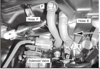
(16) Install the 6mm joint pipe and 6mm hose to the hose F. (Dia. 17, 18)
